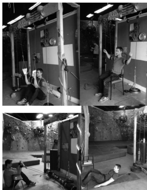
Figure 5. This shows the weighted rope and pulley systems for each prefatiguing exercise. Clockwise from top left: digit flexion apparatus, shoulder adduction apparatus, elbow flexion apparatus, and lumbar flexion apparatus.
