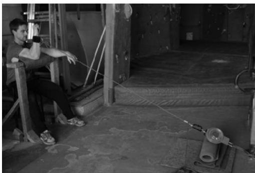
Figure 2. Elbow flexion dynamometry (forearm pronated). With an isometric contraction of the elbow flexors, the participant pulls backward against the dynamometer as hard possible for 3 seconds.
